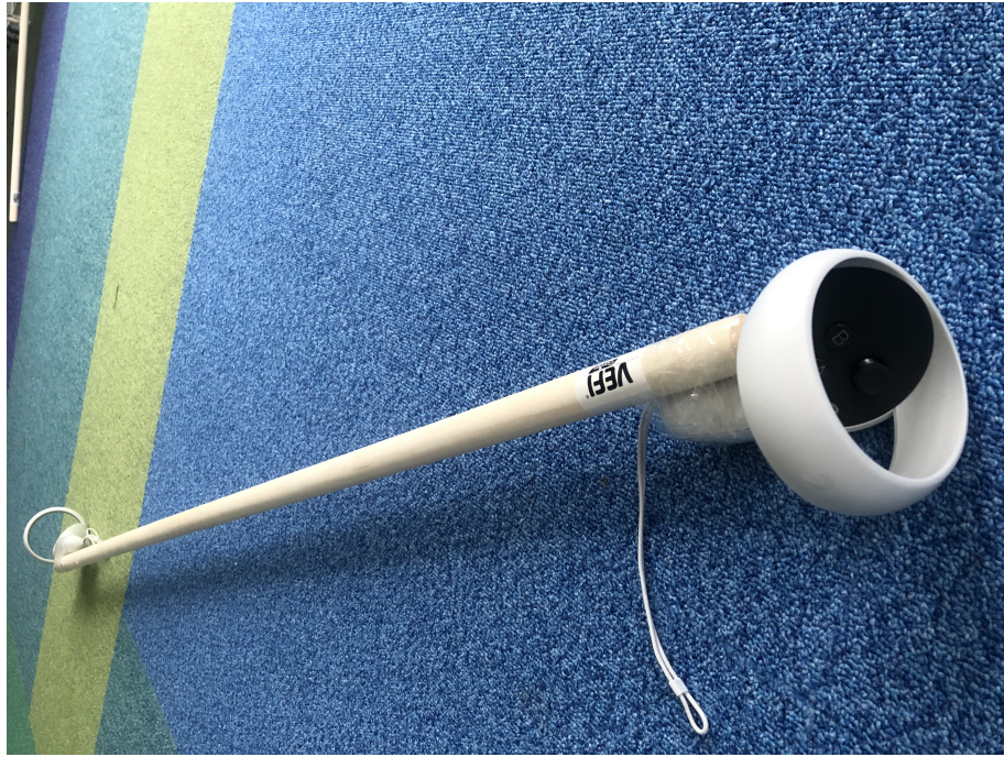
Figure 6.3: The makeshift VR staff: a wooden dowel with an Oculus Quest 2 controller taped onto each end. The motion trackers in the controllers were used as a proxy for the orientation of the staff, which the student could see in the VE.
