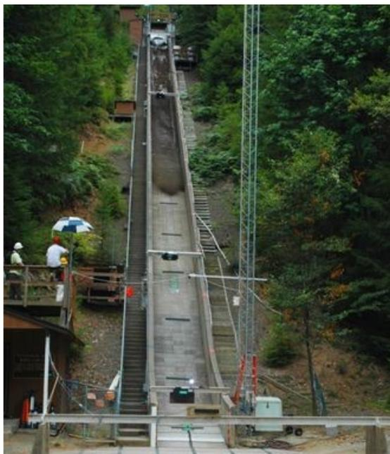
Figure 2.5: Photograph of the USGS debris flow flume during a test (photograph taken from George and Iverson, 2014).
