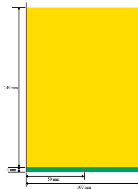
Fig. 21. Geometric configuration of the case consisting of a water column of height = 140 mm and width = 100 mm resting on a flexible plate of height = 4 mm. A vertical initial crack line (red colour) of length = 1.8 mm is located at the middle of the flexible plate. (For interpretation of the references to colour in this figure legend, the reader is referred to the web version of this article.)
