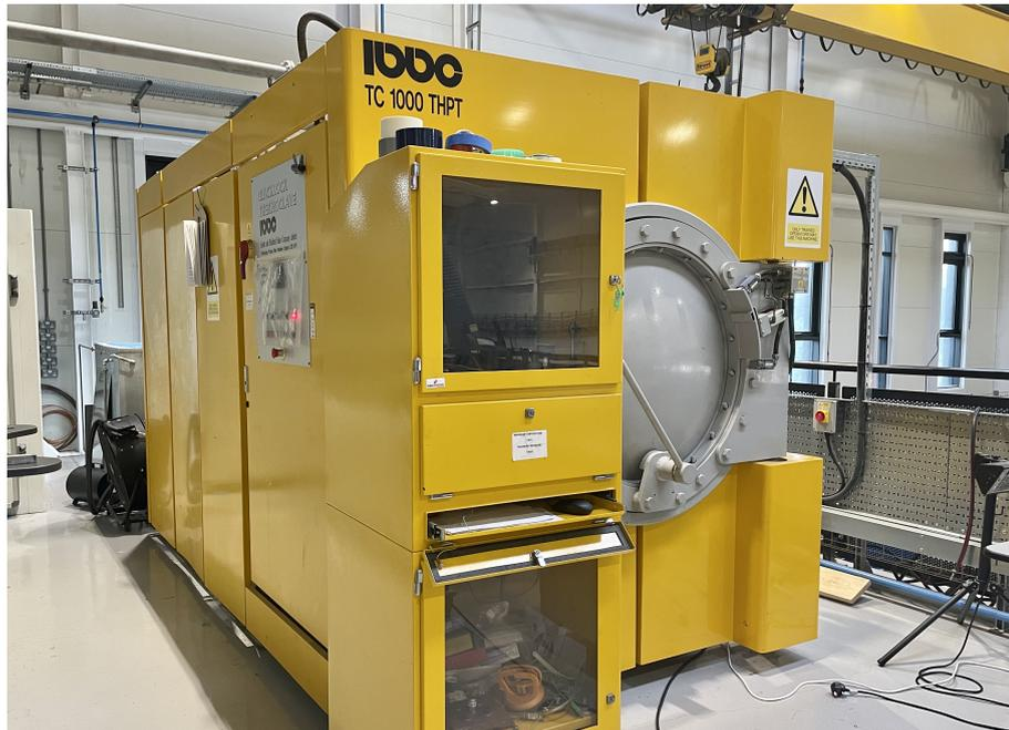
Figure 1.1: Autoclave in the composites manufacturing laboratory at University of Nottingham
