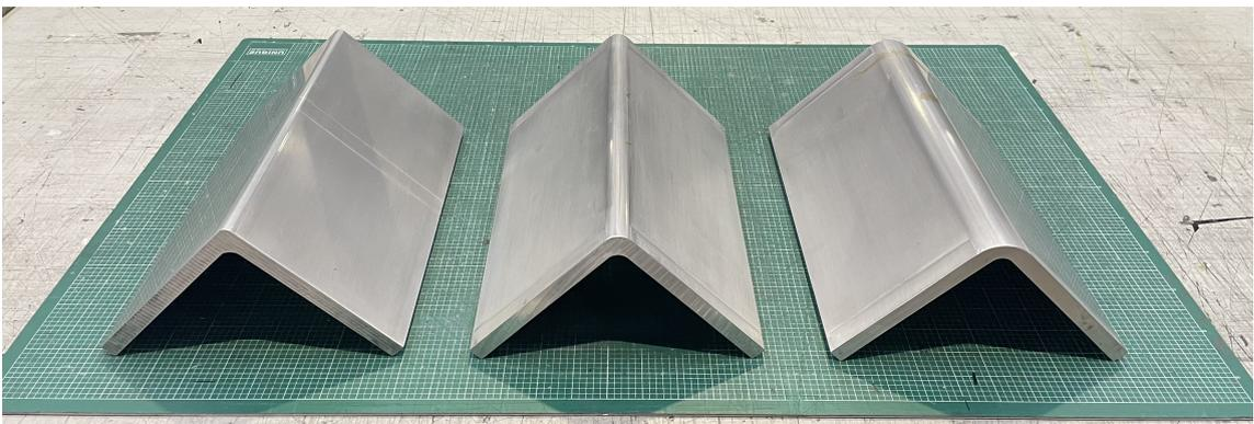
Figure 6.1: Aluminium tools with 0.25/0.5/1.0 inch radius at the curvature
