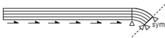
Figure 6.19: Boundary conditions for tool-part interaction analysis of the L-shaped laminates
