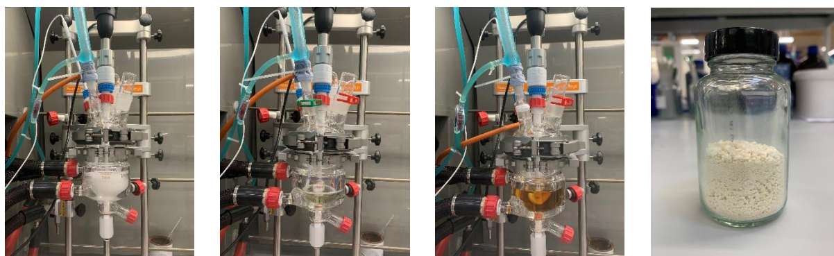
Figure 20: Large scale reductive amination – A. Reaction set up using jacketed vessel. Before addition of silane and amine. B. Reaction mixture after amidation phase complete. C. Reaction mixture after reduction phase complete. D. Benzene sulfonic acid salt of the product
