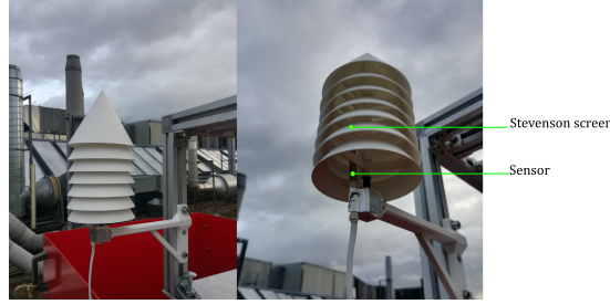
Figure 3.9: 3D printed Stevenson screen used to shield the PT100 sensor for the ambient air temperature measurement.
