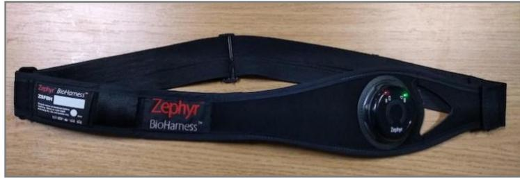
Figure 5-7 Zephyr BioHarness for heart data
