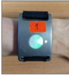
Figure 5-6 Q Sensor for EDA data
