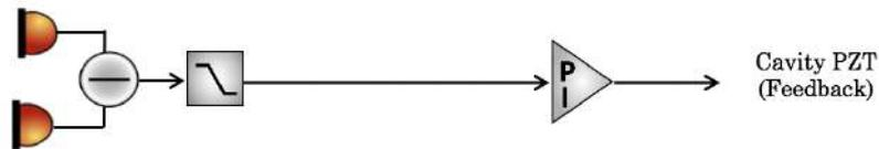
**Figure 4.13:** Locking setup to lock the MIM cavity via balanced signal.
