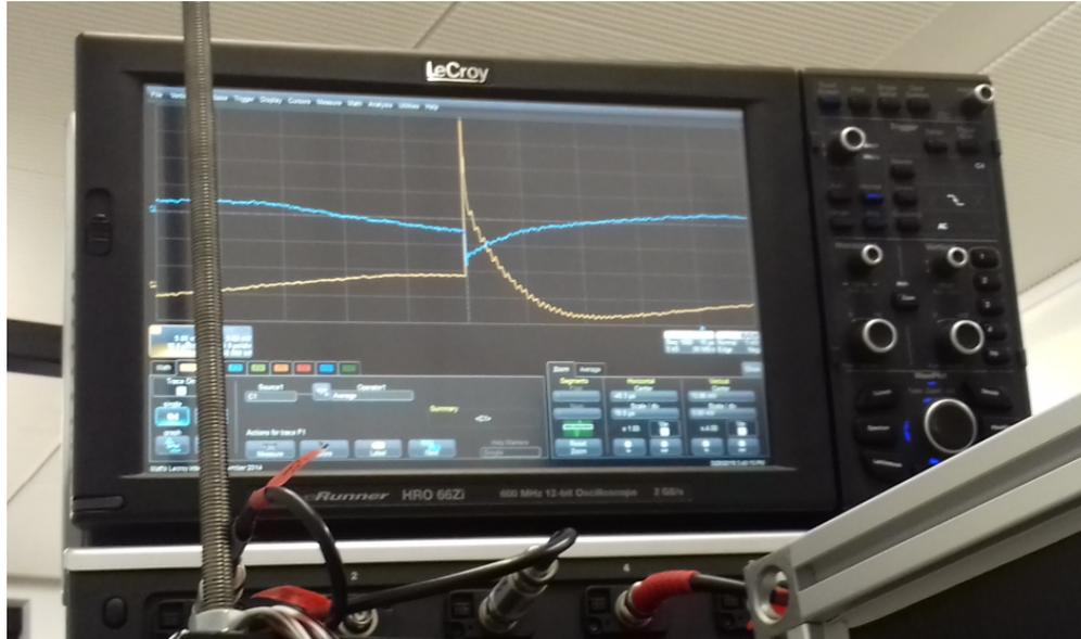
Figure 4.7: Laboratory image of an oscilloscope showing a trace from an EBL fabricated GNR detected along the length (yellow) and the width (blue). It can be seen that the rod turned off when it was detected along the width.
