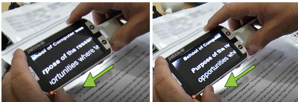
Seg. 4.5b: Framing portable electronic magnifier over printed sheet
