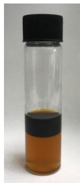
Figure 7-2 Emulsified solvent-oil blend with 20 wt. % 2-Octanol
