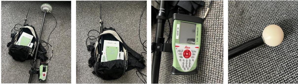
Figure 8: Images of the *Leica GS10* GNSS receiver with a *CS10* controller and rounded base used in the field.
