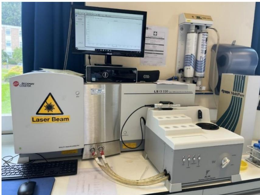
*Figure 9: The LS 13 320 Laser Diffraction Particle Size Analyzer used to determine sand sediment grain size.*
