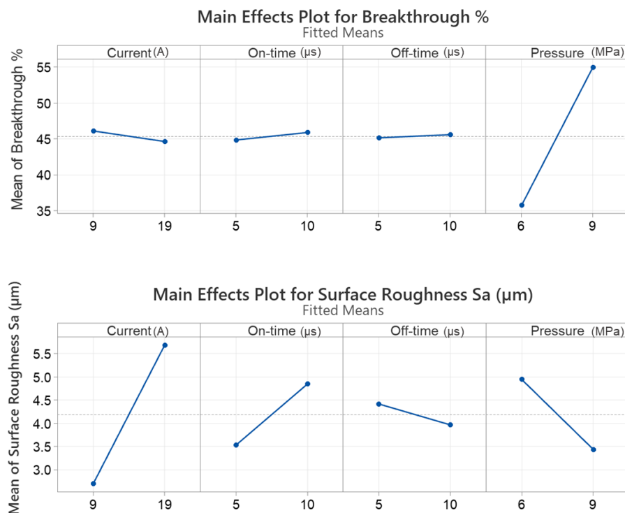
Figure 25. Main effects on breakthrough percentage and surface roughness of current, on-time, off-time, and pressure.
