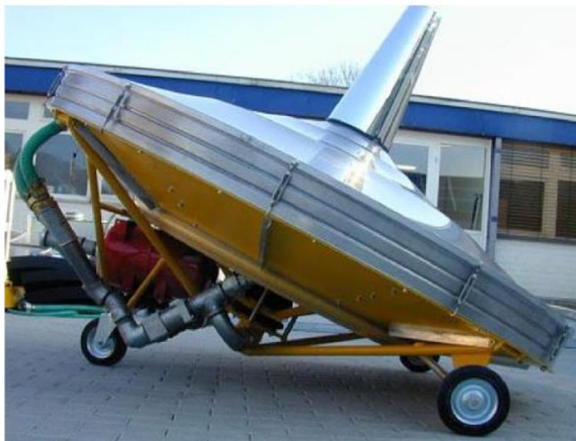
Figure 3.21: SUNPULSE Stirling System [45]
