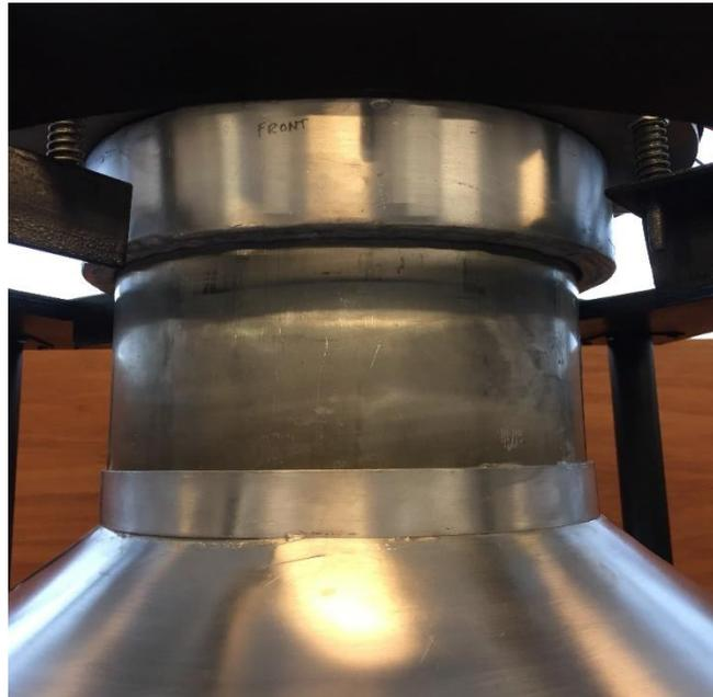
Figure 5.13: Water jacket cooling design
