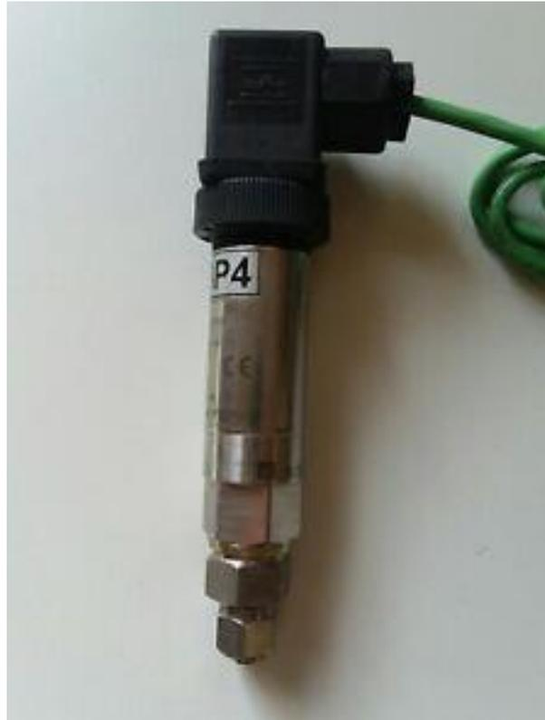
Figure 6.5: The UNIK5000-PTX5072 pressure transducer
