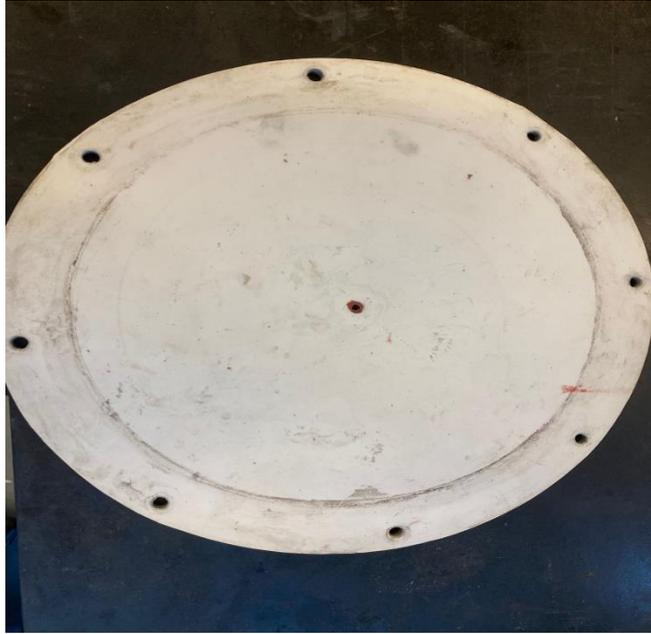
Figure 5.6: Diaphragm of engine power piston
