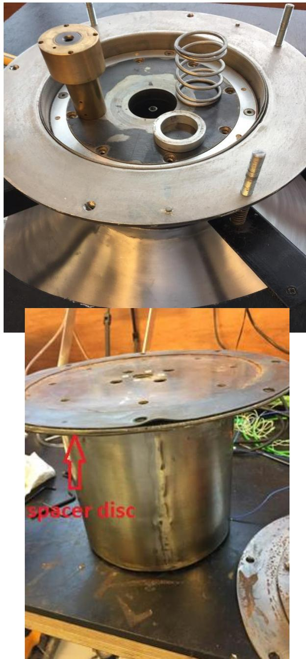
Figure 5.4: The combined displacer with the cylinder
