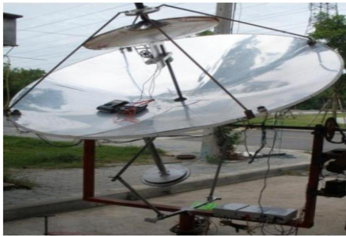
Figure 3.15. 2-stage parabolic dish-Stirling engine
