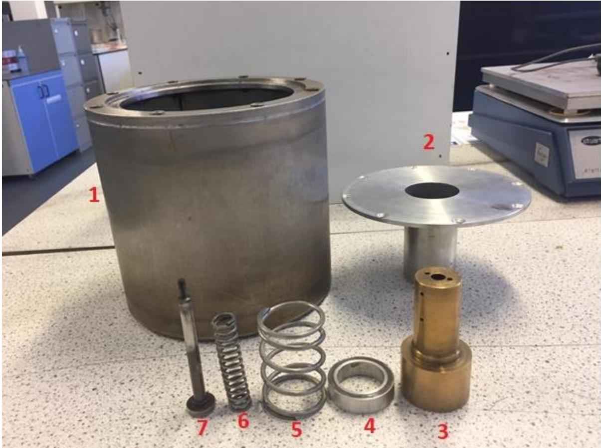
Figure 5.3: The components of the displacer
