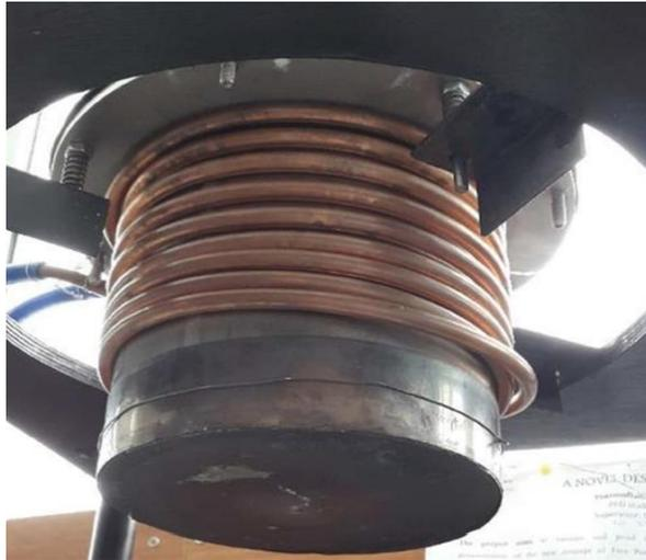
Figure 5.8: Cooling coil design
