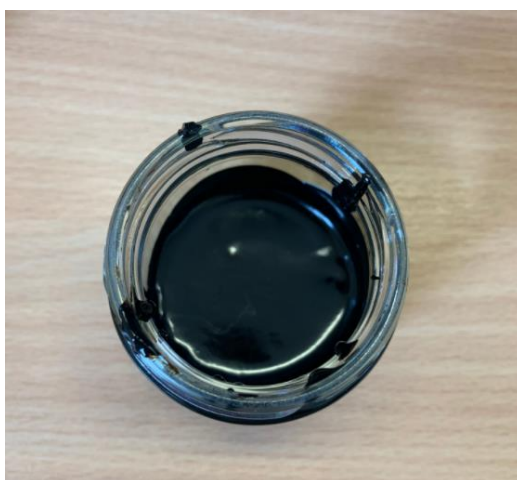
Figure 26: Pyrolysis product obtained at 300 °C after 5 hours from the untreated BFO.
