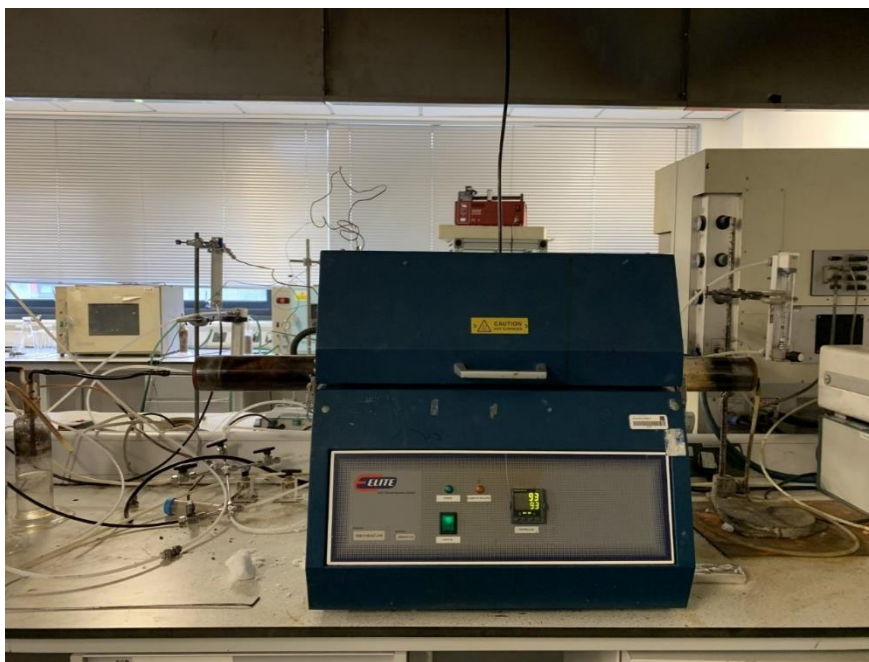
Figure 16: Pyrolysis equipment using a high-temperature horizontal furnace (HTF).
