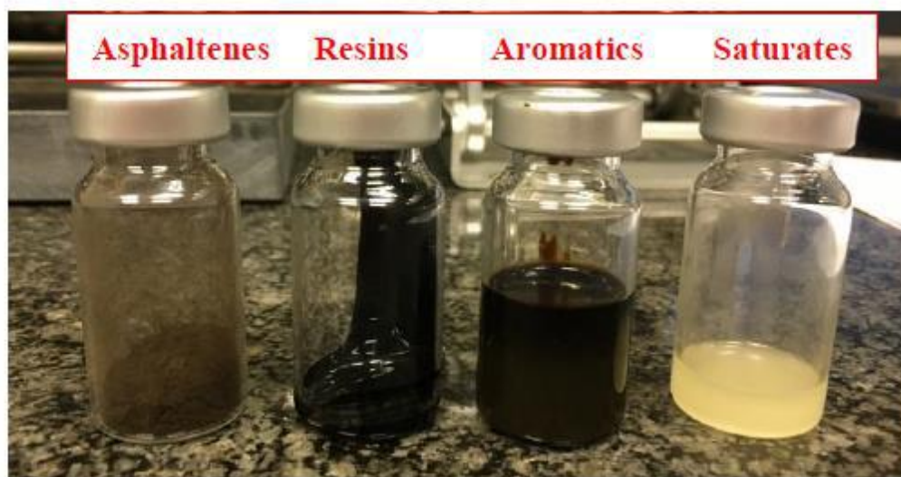
Figure 7. Bitumen fractions, obtained through SARA analysis (Jimenez del Barco Carrion, 2017).
