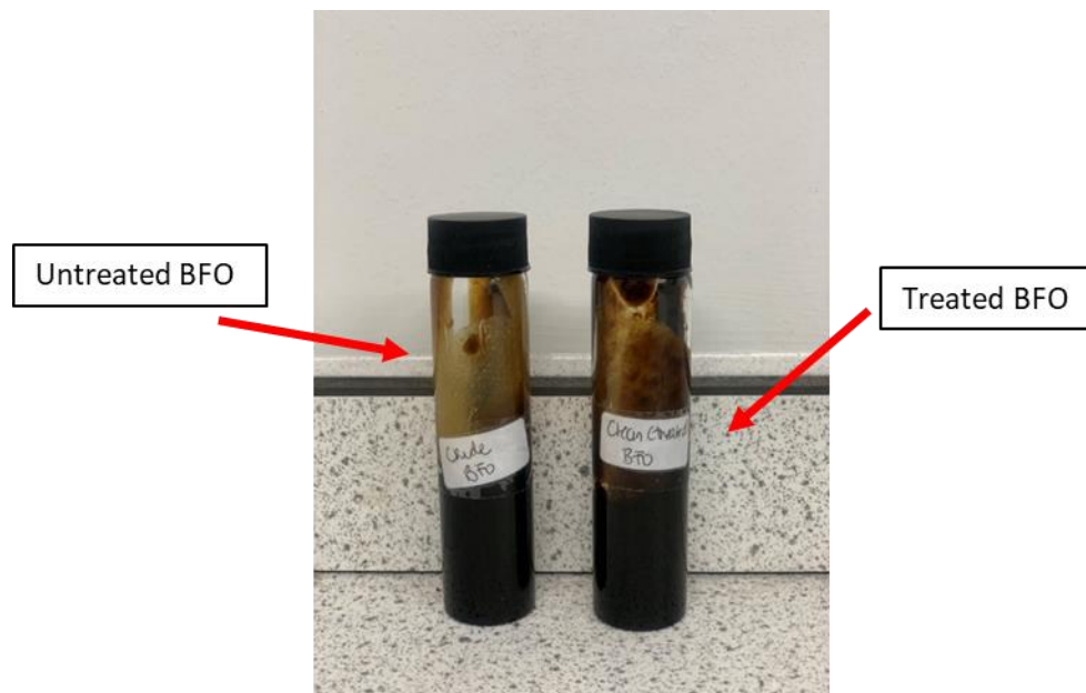
Figure 1: Biofuel Oil, referred to as BFO. The BFO has been treated with 2% water and 1% phosphoric acid to strip out metals and other solids. According to Argent Energy, this treatment is used to make the BFO more fluid at ambient temperature.
