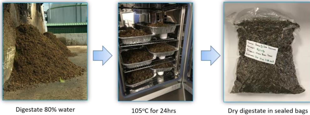
**Figure 14.** Crop digestate samples preparation.
