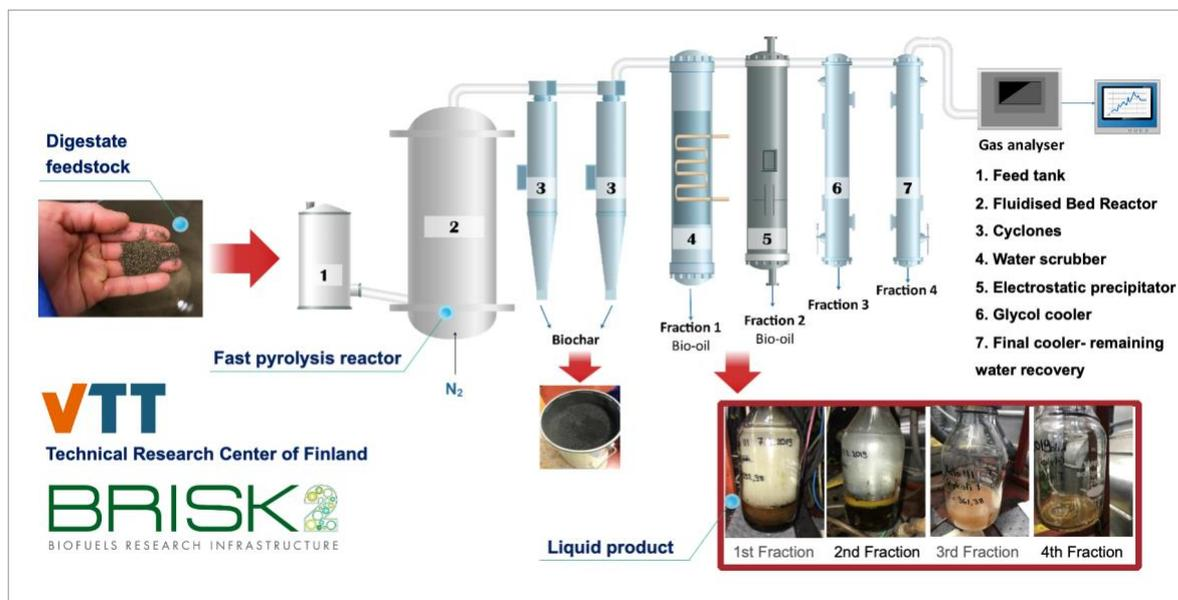
**Figure 23.** General diagram of fast pyrolysis system in VTT, using crop digestate.
