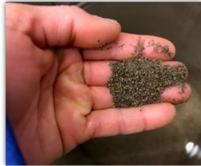
**Figure 21.** Digestate in particles 0.5-0.9 mm
