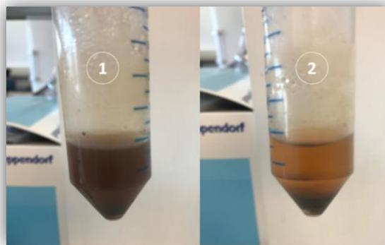
**Figure 17.** Difference between two hydrolysis processes implemented to determine carbohydrate levels in crop waste and digestate: (1) strong hydrolysis (2) weak hydrolysis
