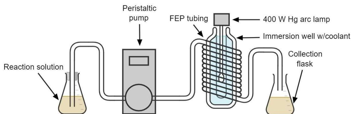
Figure 8: Diagram of FEP reactor setup.
