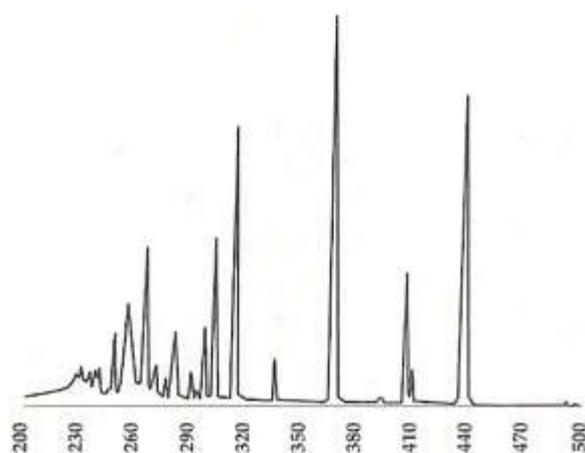
*Figure 3: An example of the emission spectrum of the medium pressure 400 W Hg arc lamp from Photochemical Reactors Ltd. Image reproduced with permission from Photochemical Reactors Ltd.*
