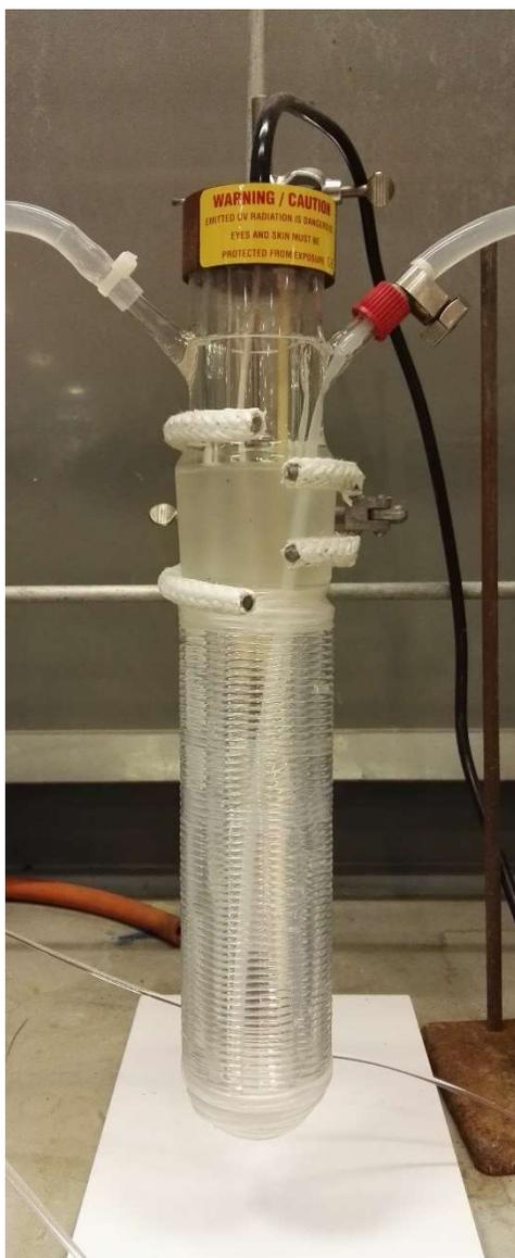
*Figure 4: Close-up of reactor, showing the immersion well wrapped with coils of FEP tubing.*
