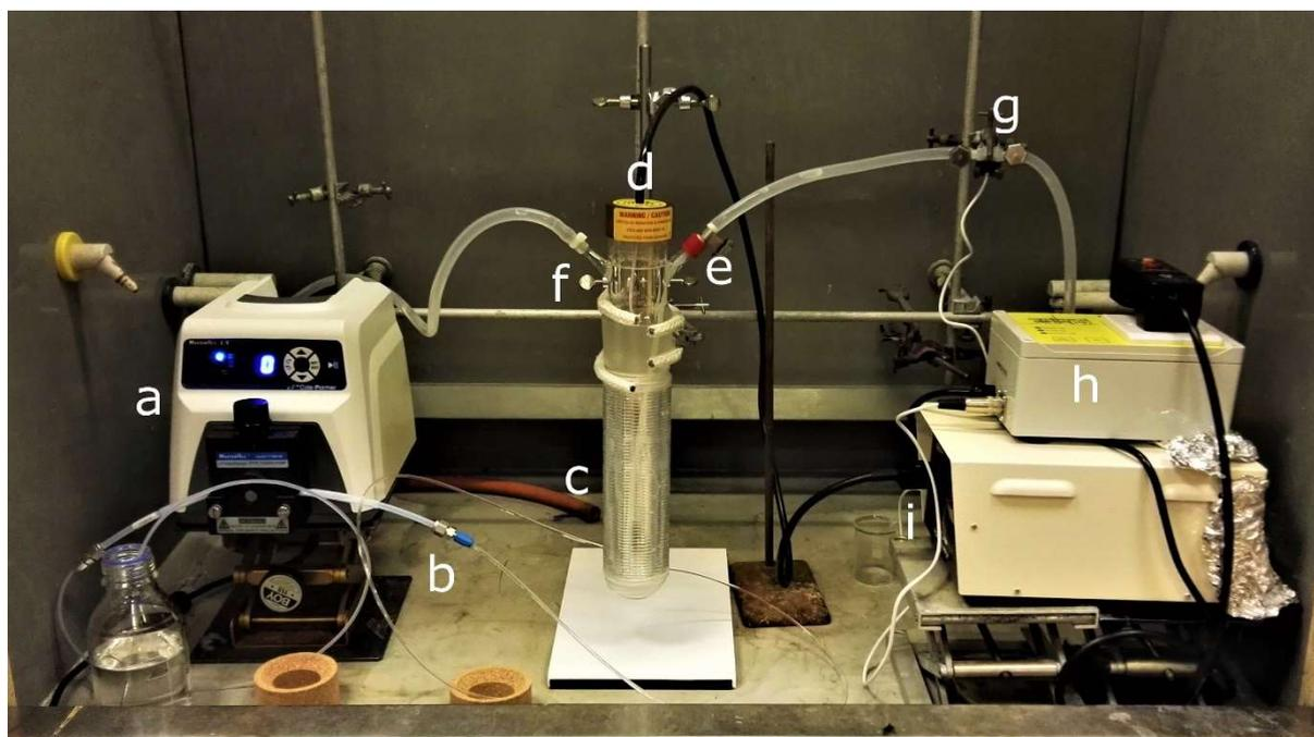
*Figure 5: Reactor set up. a) peristaltic pump, b) PTFE to FEP union (contains O-Rings), c) Reactor coil, d) 400 W Hg lamp, e) water coolant input, f) water coolant output, g) coolant water flow monitor, h) power cut-off control, i) 400 W power supply.*
