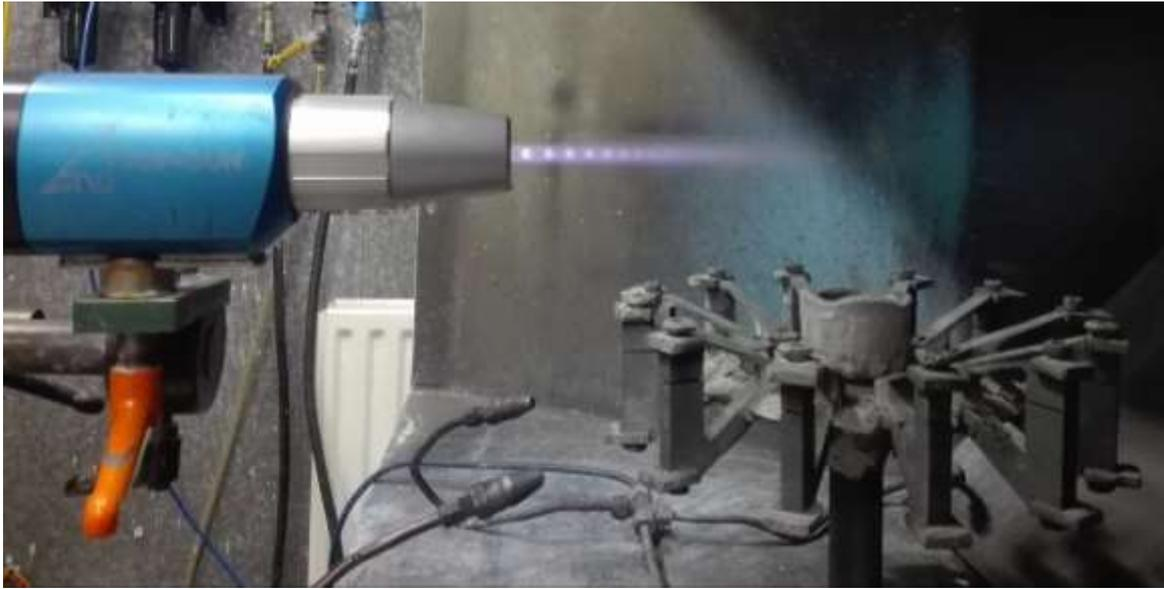
*Figure 81: Photo of the spraying setup where the spray gun (left) is visible along with the sample carousel (right)*
