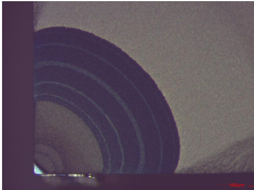
Fig. 4.20: RR1000 Fracture Surface - Symmetrical - Beach Mark Plan
