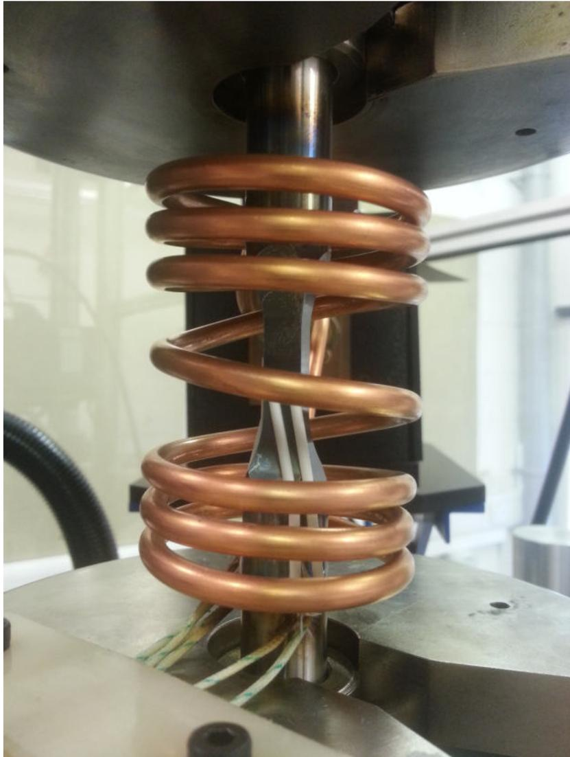
*Fig. 3.4:* Induction Coil and Thermal Calibration Specimen
