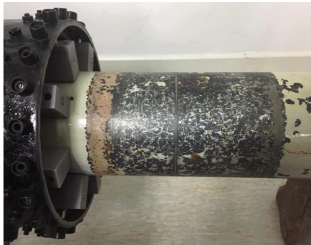
Figure 51: Oil and gas pipe with 1.0mm or 1.5mm defects
