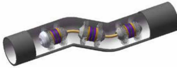
Figure 7: An ultrasonic tool navigating through a pipeline.
