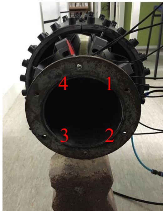
Figure 19: Oil and gas pipeline with quadrant number for transducer collars
