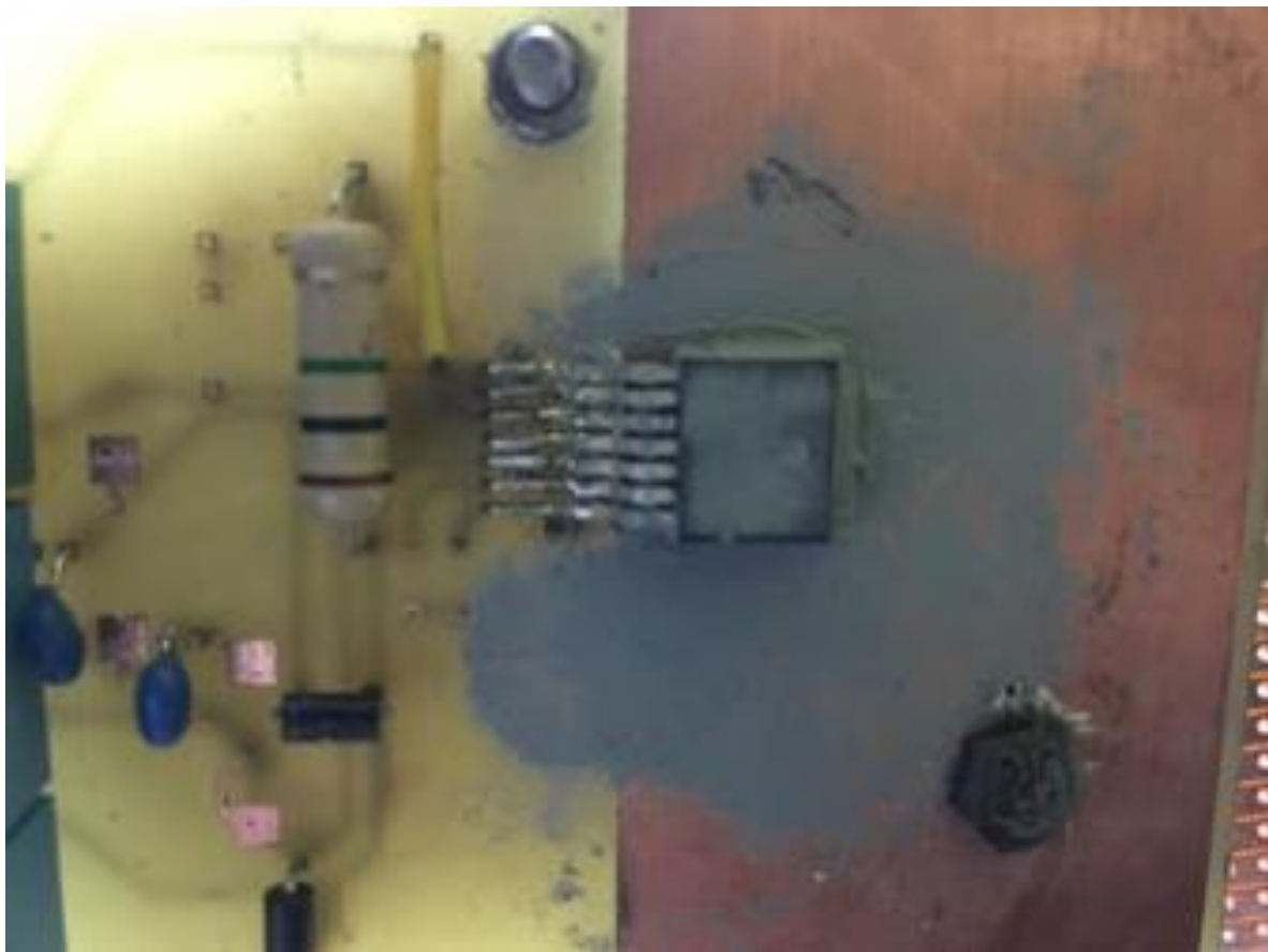
Figure 16: PA240cc Operational Amplifier with copper pour
