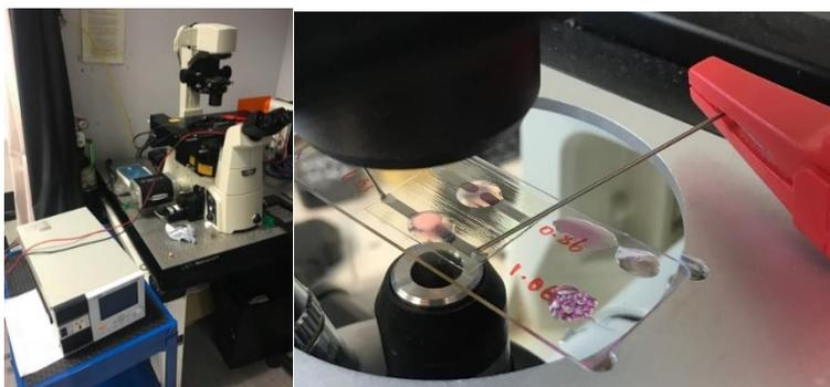
**Figure 2-3 Wire growth set up, using optical microscope, high voltage stimulator (HVS), Ag paint contacts and needle electrodes.**
