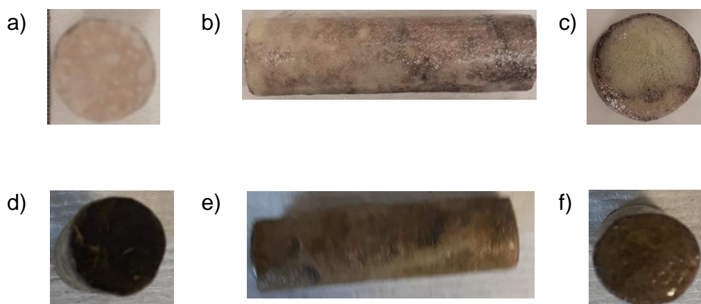
Figures 4.4: Images 4.4a-f show a bolus used in the preliminary trial. Images 4.4 a-c showed the bolus prior to administration. 4.4a shows the radial view of the open end of the bolus, b: the axial view of the bolus and c: the radial view of the sealed end of the bolus. Images 4.4 d-f display the same bolus once retrieved after ingestion, with the images in the same order.
