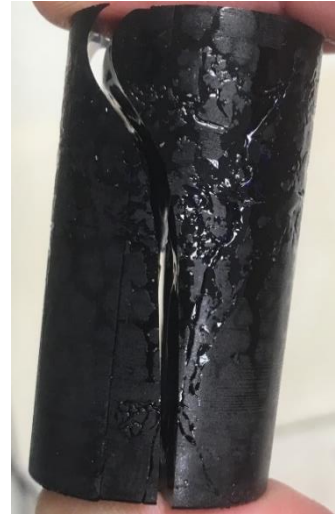
Figures 2.15 a-f: Images taken of the cooled hollow billets after following different annealing regimes (outlined in Table 2.3), once removed from the mould.
