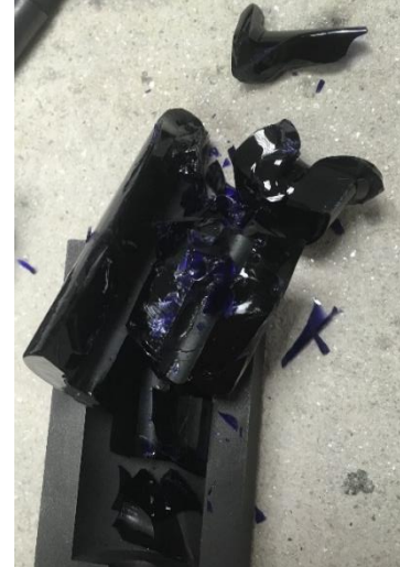
Figures 2.15 a-f: Images taken of the cooled hollow billets after following different annealing regimes (outlined in Table 2.3), once removed from the mould.
