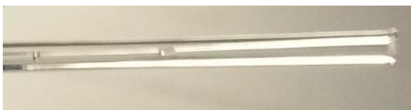
Fig. 39 - Liquid Visible in the Connector Removed from Between the Guard and Analytical Columns. This was presumed to be IL that was carried through the guard column by the carrier gas and deposited in the wider connector where the gas could more readily flow around it.
