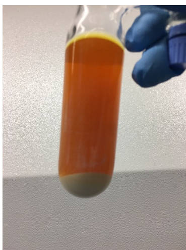
Figure 2-14. Picture showing the pale off-white precipitate silver iodide by-product, following the reaction of 16 with silver oxide. Under the same conditions treatment of 10 with silver oxide produces a much lower quantity of pale yellow \text{AgCl} precipitate, with a significant proportion of unreacted silver oxide remaining.
