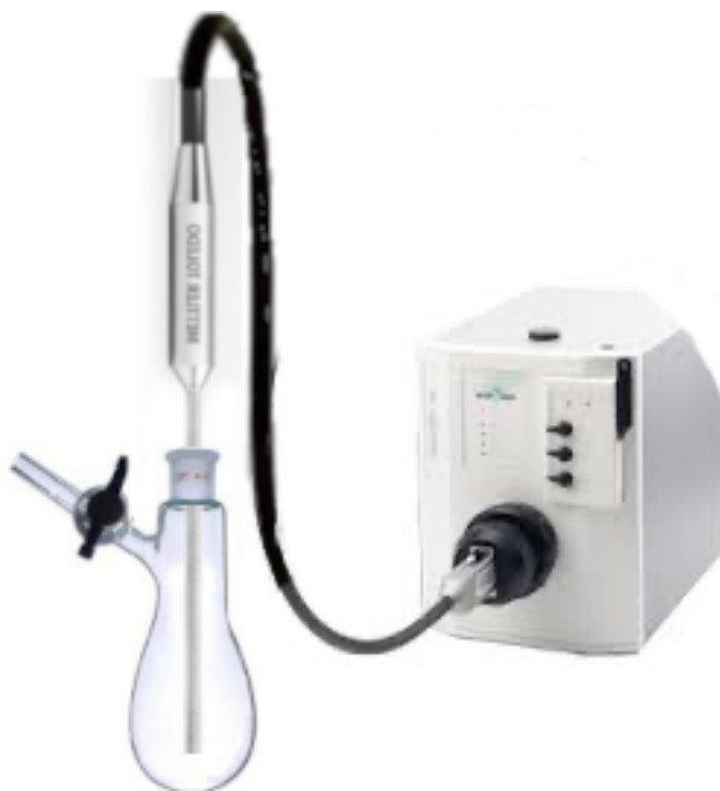
Figure 3-12: Schematic setup for ReactIR measurements. Diamond ATR probe, connected to a ReactIR 15, inserted into a Schlenk flask, under a positive pressure of argon.
