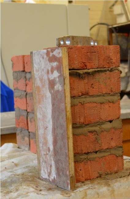
Figure 4.2: Preparation of the masonry wallettes
