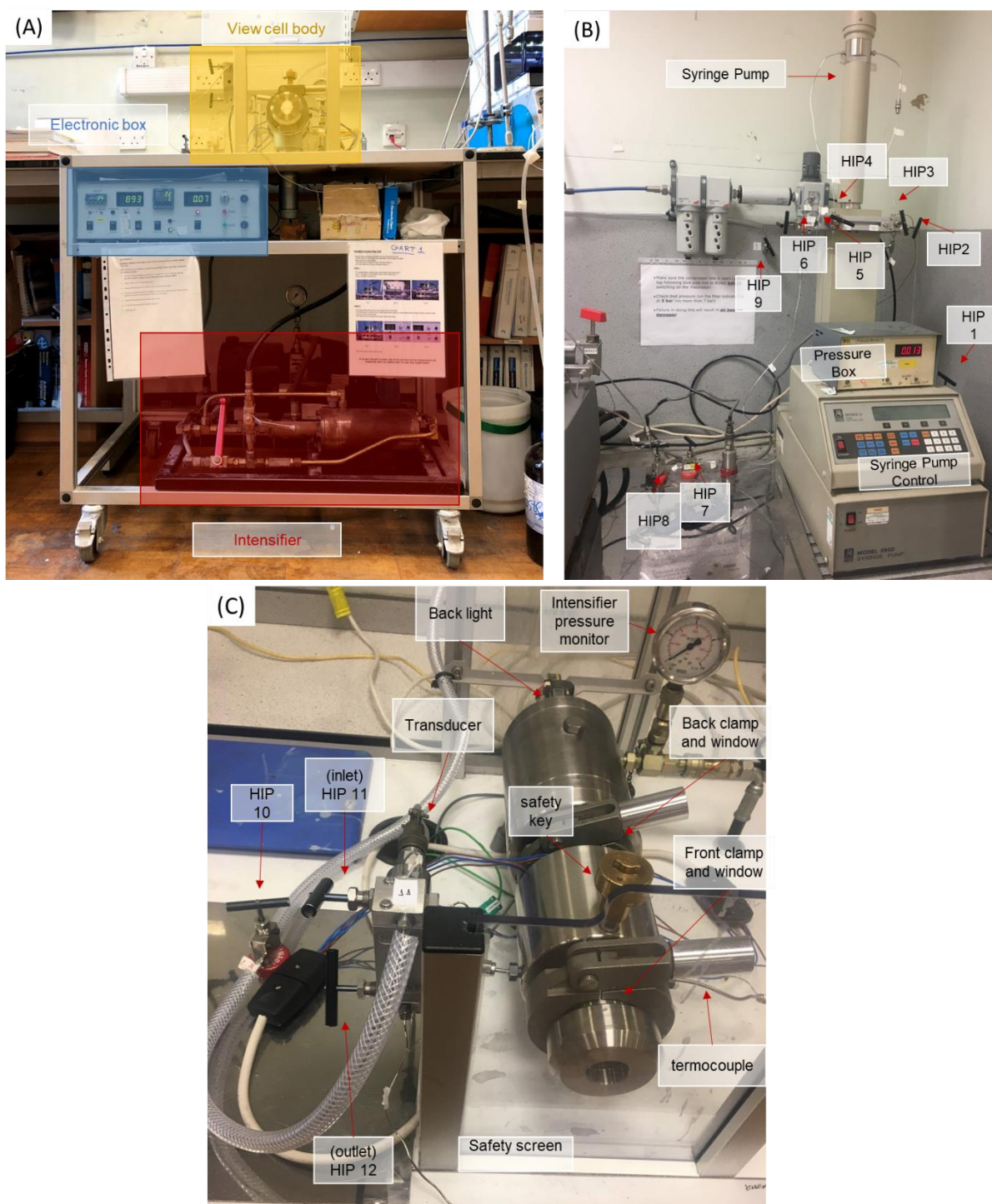
Figure 10 – Photographs of the high-pressure variable volume view cell rig setup. (A) Main rig – with the intensifier, electronic box and view cell body; (B) Syringe Pump set up for the view cell feeding; (C) close up of the view cell body – showing the inlet, outlet, internal thermocouples, safety key, clamps, transducer, safety screen, back light and monitor for the intensifier pressure.
