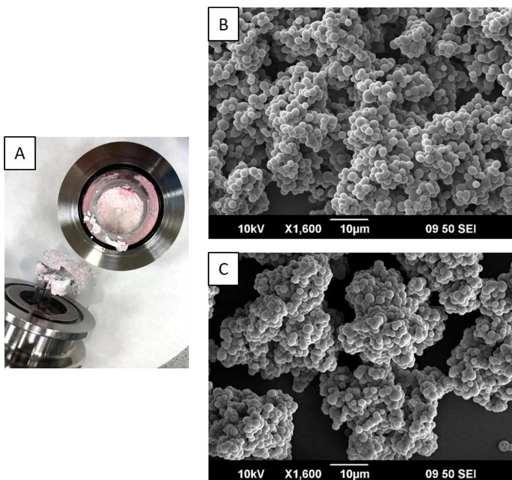
Figure 24 - Picture of final product obtained as a light pink powder for E2.8 (A); and SEM picture of E2.8 (B) and of E2.9 (C), both obtained using a JEOL 6060LV SEM at accelerating voltage of 10 kV and at 1600x magnification.
