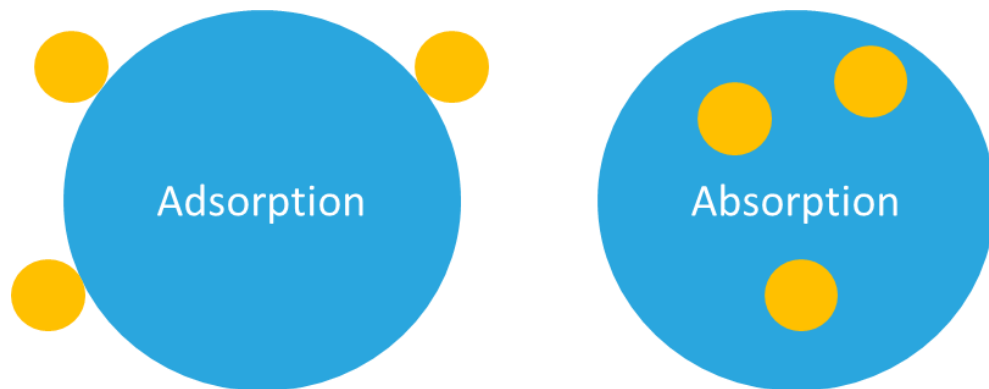
Figure 2.13 Schematic description adsorption and absorption.
