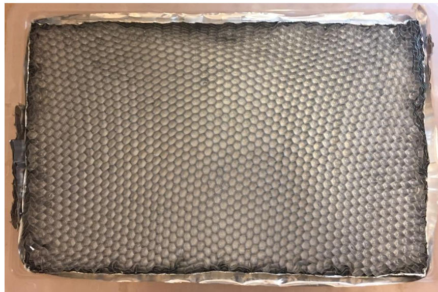
Figure 5.4 Metal honeycomb structure with PCM.
