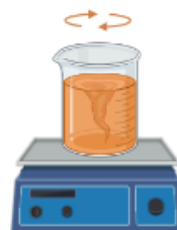
Figure 6.32 Magnetic stirrer schematic function.
