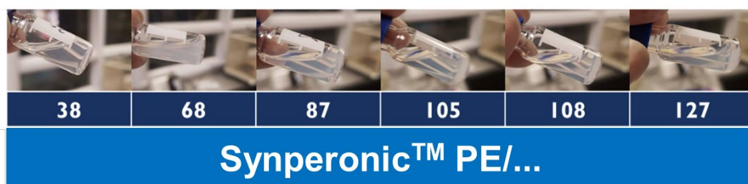
Figure 3.3.8: Photographs of sample following extrusion of hexasomes produced using various flake Synperonic™s. w/w/w ratio (mg:mg:mg) of Cithrol™: Synperonic™: Water was constant at 6:1:113. Formulations were extruded using an Avanti mini-extruder with a 200 nm membrane.
