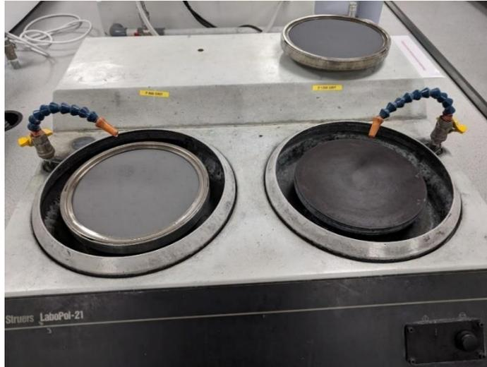
**Figure 3-4 Polishing Apparatus**
