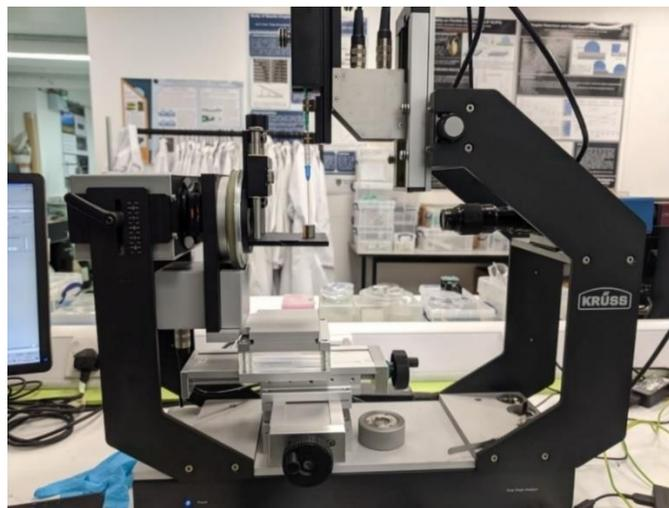
**Figure 3-3 Krüss contact angle measuring apparatus**
