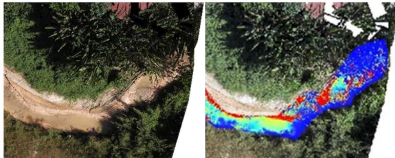
**Fig. 4.5** Effects of riparian vegetation on the estimation of SSC. The left image shows the orthomosaic section of the upstream tributary which is greatly covered by vegetation while the right image is the SSC map derived from the orthomosaic.
