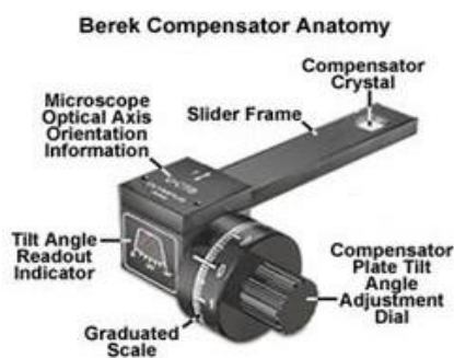
Figure 2.12 Berek compensator. It clearly shows microscope optical axis orientation, compensator crystal, Graduated scale, Tilt angle indicator, Compensator plate tilt adjustment dial This figure was adapted from the website [88]
