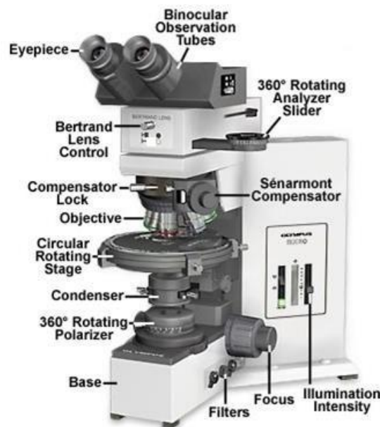
Figure 2.11: BX51 Polarising light microscope. This figure was adapted from the website[87]. Labels are clearly demonstrating the parts of the microscope- Where the polarised is positioned, circular rotating stage, condenser, compensator lock, eyepiece.
