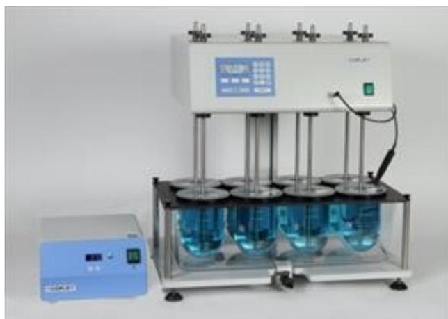
FIGURE 3.17: Copley scientific Dissolution Test Dis8000, image from Copley scientific's catalogue [204]
