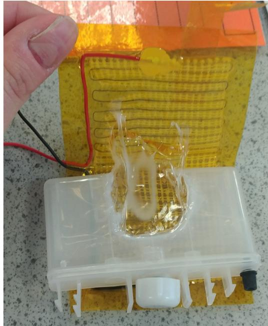
FIGURE A.5: Damage to Dimatix cartridge after heating experiment
