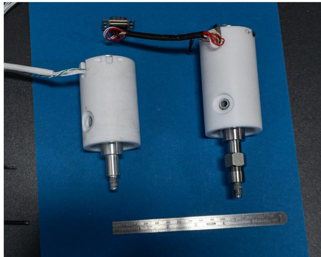
FIGURE 2.7: Comparison between the original hot-melt reservoir from Meyer Burger (Right) and our redesigned version (Left).
