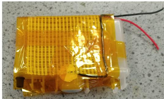
FIGURE A.3: Dimatix Material Cartridge surrounded by a heating pad.
