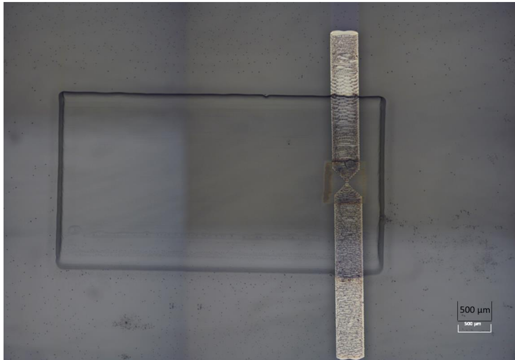
Figure 6.13 Optical microscope image of printed drain electrode, source electrode, semiconductive channel and dielectric film on the glass slide.
