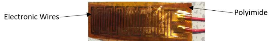
Figure 3.7 Thin film heater with a power of 10W.
