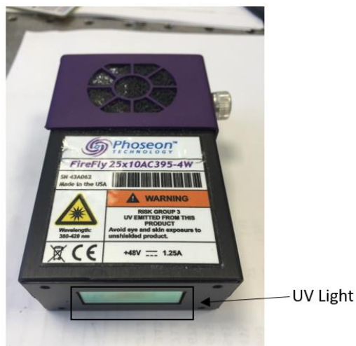
Figure 3.9 Photo of the UV illumination reaction unit.
