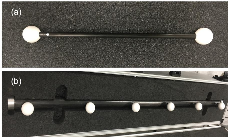
Figure 6.3: Artefacts used for the verification test. (a) A ball bar and (b) a ball beam.
