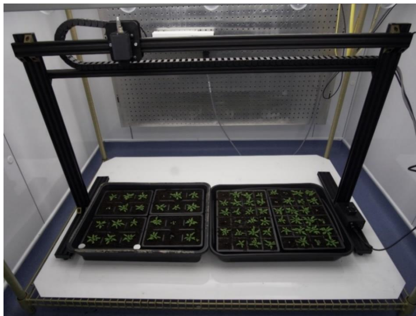
Figure 5.1: Bespoke HTP thermal imaging robot, in situ .
