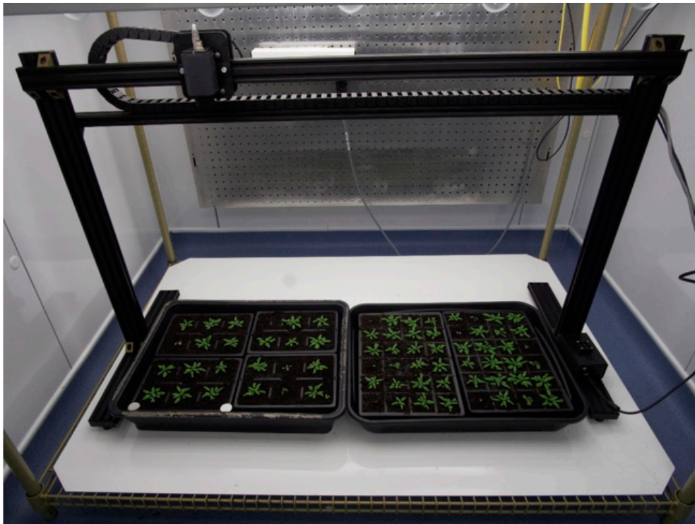
Figure 2. Thermal Imager. For scale, the drive rail is 1.2 m in length.
