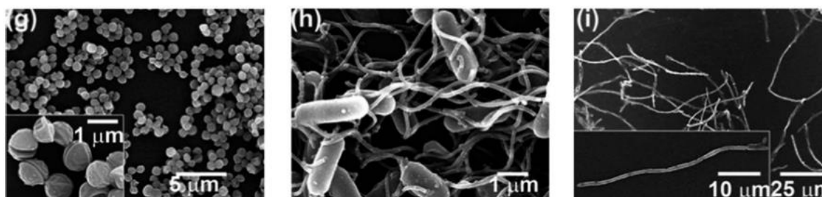
Figure 1.4: Particles fabricated using soft templates. SEM images of g) Cocci templated particles h) E. coli templated particles i) Mildew fungus templated particles. Adapted from reference 178
