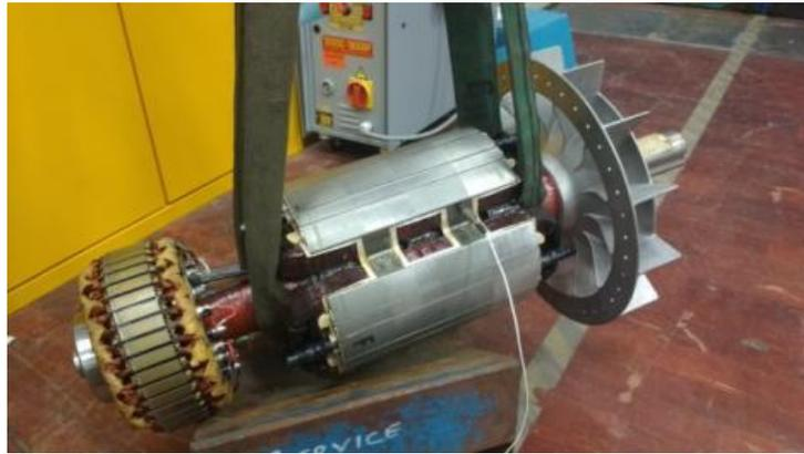
Figure 3.3: Suspended F Core Rotor. Accelerometer positioned for torsional mode acquisition from the core
