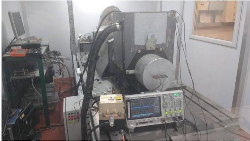
Figure 4.6: UC22F generator and electric motor test rig prepared for steady state and three phase short circuit experimental tests
