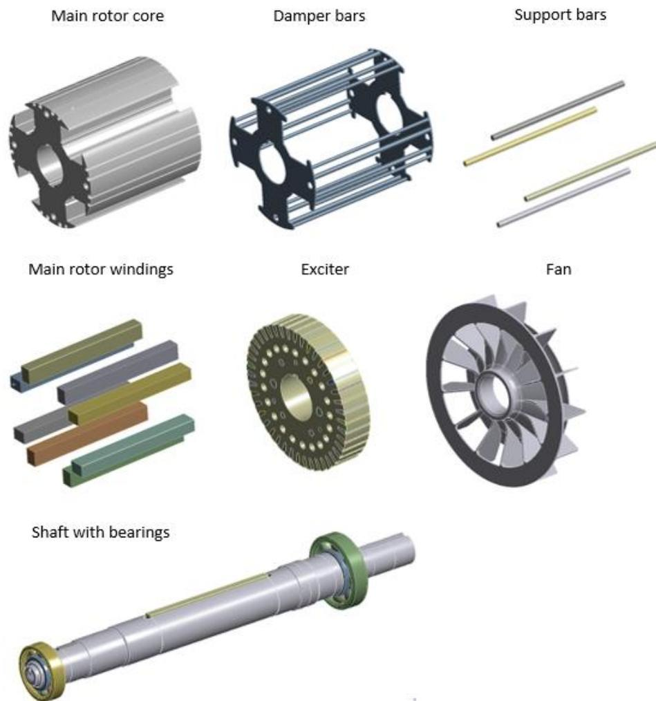
Figure 2.16: Generator rotor components.
