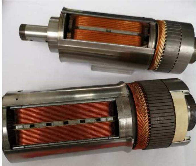
Fig. 52 Cross sectional view of commercial WFSGs implemented on aircraft
