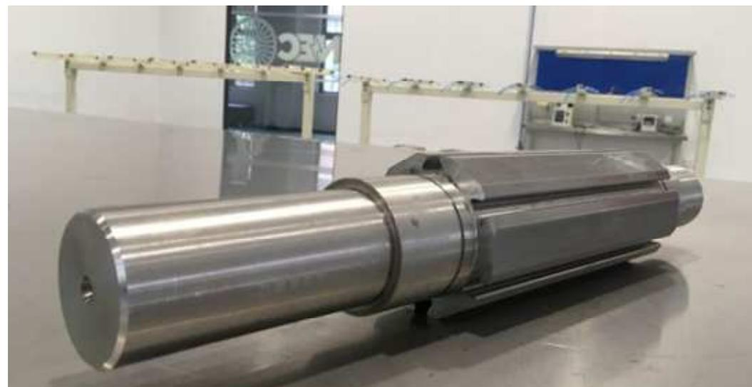
Fig. 101 A customized shaft for a WFSG designed in chapter 5.3.3
