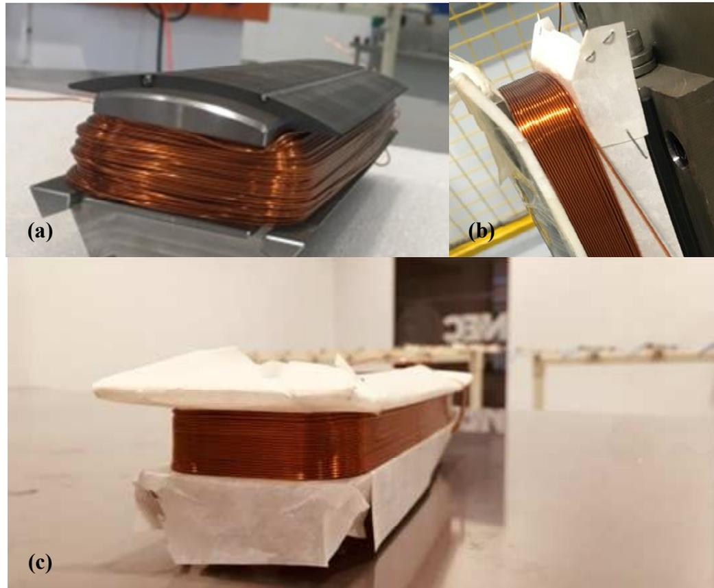
Fig. 104 a) first rotor core assembly b) modified winding process c) outcome of final rotor core outlook
