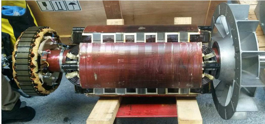
Fig. 70 A complete rotor core (Courtesy Cummins Generator Technologies)
