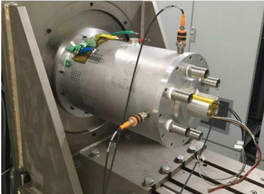
Fig. 109 The final assembly for a WFSG prototype
