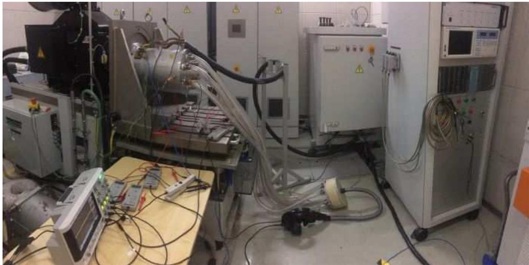
Fig. 111 Overall rig setup for a WFSG testing
