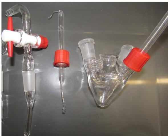
**Figure 4.2.** Five-necked cell with large central neck for RDE experiments, showing from left to right gas inlet tap, Pt coil electrode and cell with Ag wire electrode.
