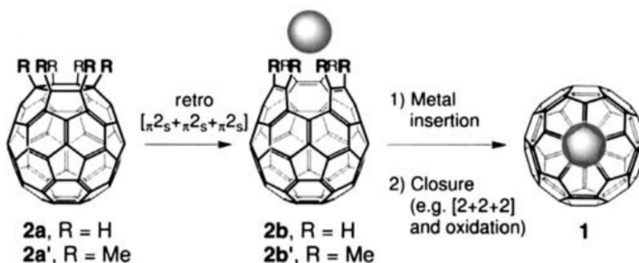
Figure 4.1. Conceptual procedure proposed by Rubin et al. for the opening and closing of a C 60 fullerene to form endohedral metallofullerenes. 21
