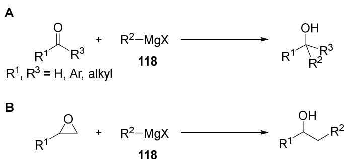
Scheme 47 Alcohol synthesis using Grignard reactions. A – Reaction between carbonyl-containing compound and Grignard reagent 118 . B – Reaction between epoxide and Grignard reagent 118
