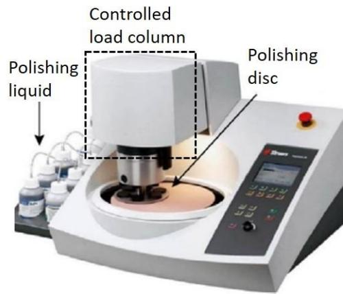
*Figure 30. Basic structure of the Struers LaboSystem Tegramin machine*
