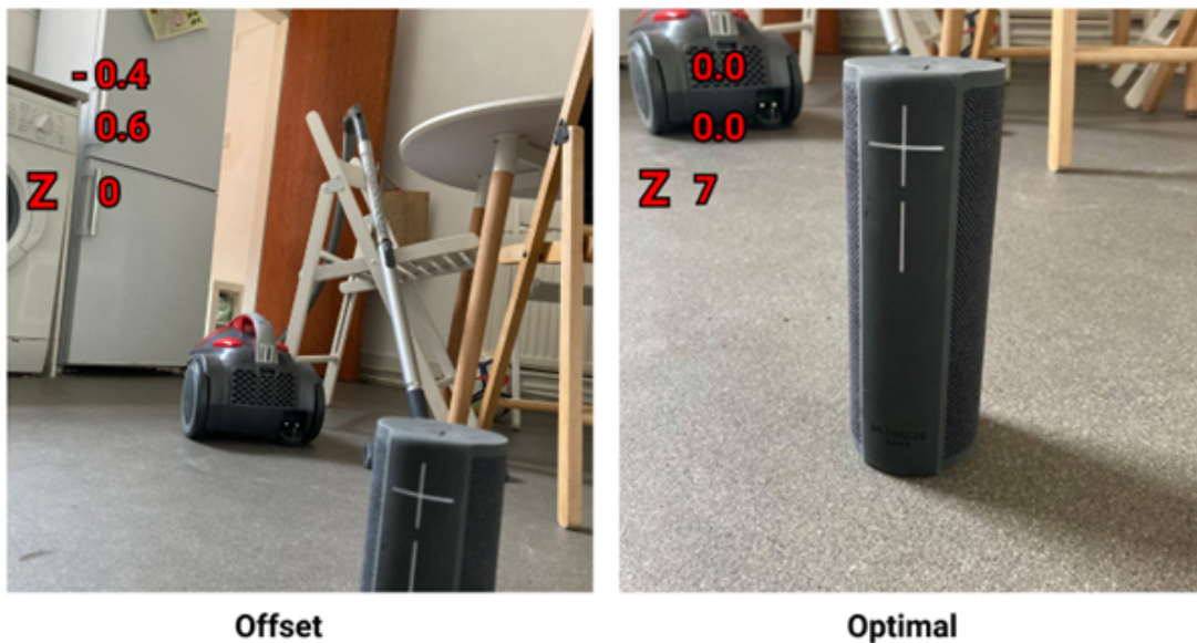
Figure 3.1: An example of the annotated ground truths generated for the network. Vertical arrows represent tilt direction and horizontal arrows represent pan; Z represents zoom. Left: The offset image, with the tilt and pan pixel offsets given in pixel values normalised between -1 and 1. The negative tilt offset means tilt the camera down, a positive pan offset means pan the camera to the right. The sign of the offset dictates the direction classification predicted by the network. The magnitude prediction is the absolute value of the pixel offset. No zoom occurs in the left-hand image as the object is too far from the centre of the image. Right: The zoom value of 7 will result in a 7x5% centre crop of the image from the edge.
