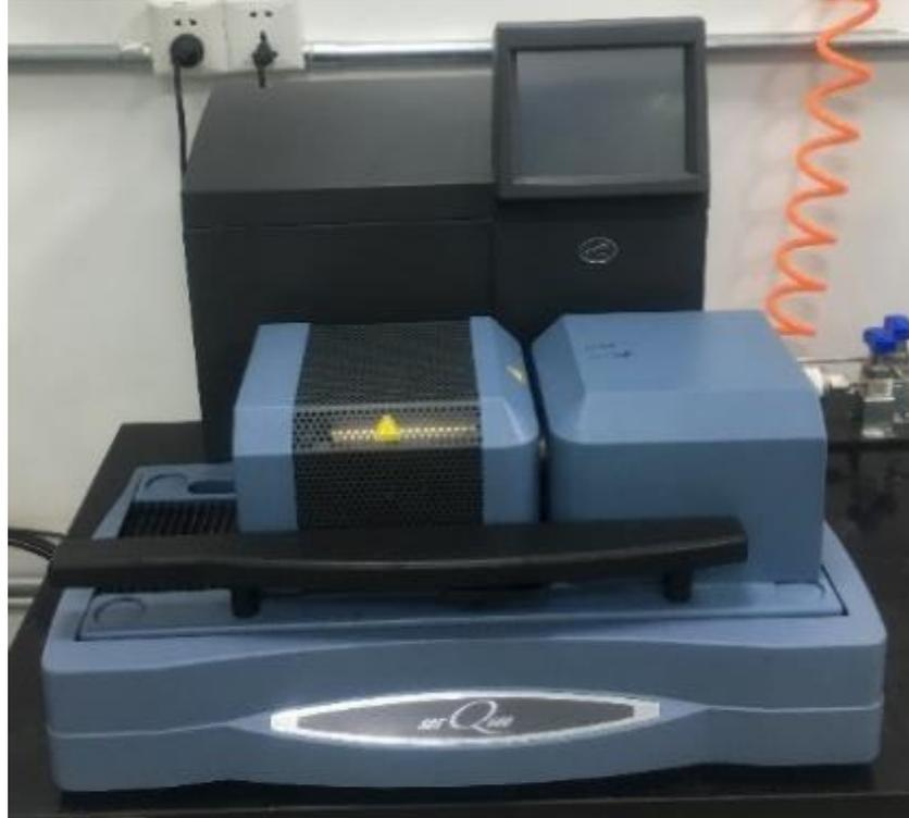
**Figure 3-2 Thermogravimetric analyser (TGA).**
