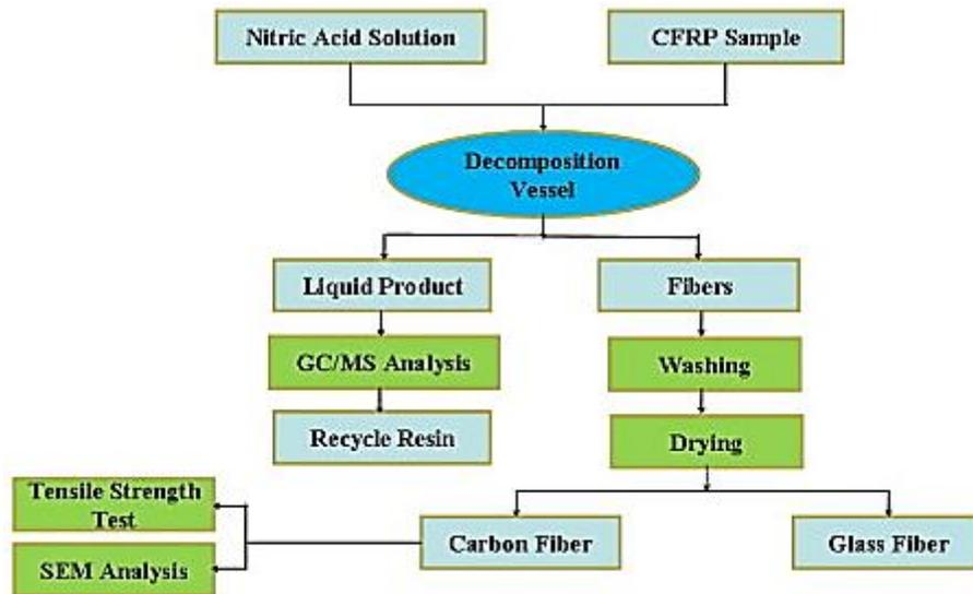
**Figure 2-2 Chemical recycling process by acids (Liu et al., 2009).**
