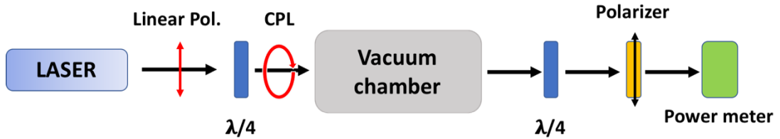
Figure 2.13. A method for measuring the Stokes polarization parameters for a circularly polarised laser pulse. The figure shows the polarizing elements that generate the Stokes parameters to be measured.
