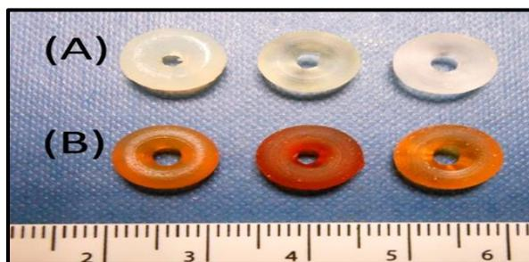
**Figure 1.6.** Images of 3D fabricated tablets loaded with (A) paracetamol and (B) 4-ASA. From top to bottom: tablets containing 35% PEGDA, 65% PEG300, 65% PEGDA, 35% PEG300, 90% PEGDA, and 10% PEG300 [132].
