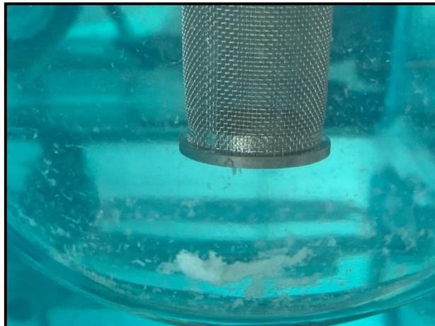
**Figure 12.** Photographic image of fabricated formulation after 10 hours in pH2 dissolution medium.
