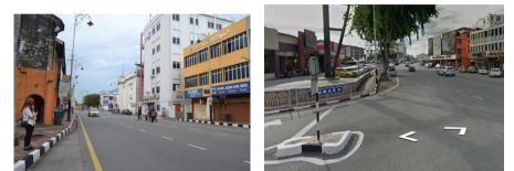
Figure 1 Pedestrian walkways along Jalan Langgar with irregular size, narrow and obstructed with street lighting posts
