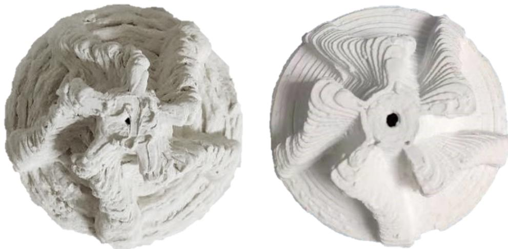
**Figure 4.17:** TiO<sub>2</sub> impeller produced before (left) and after (right) adding the boundary lubricant (Composition before: 1:0.9 - [TiO<sub>2</sub>]:[10% PEG solution] and After: 1:0.9:0.1 - [TiO<sub>2</sub>]:[10% PEG solution]:[Lubricant]).
