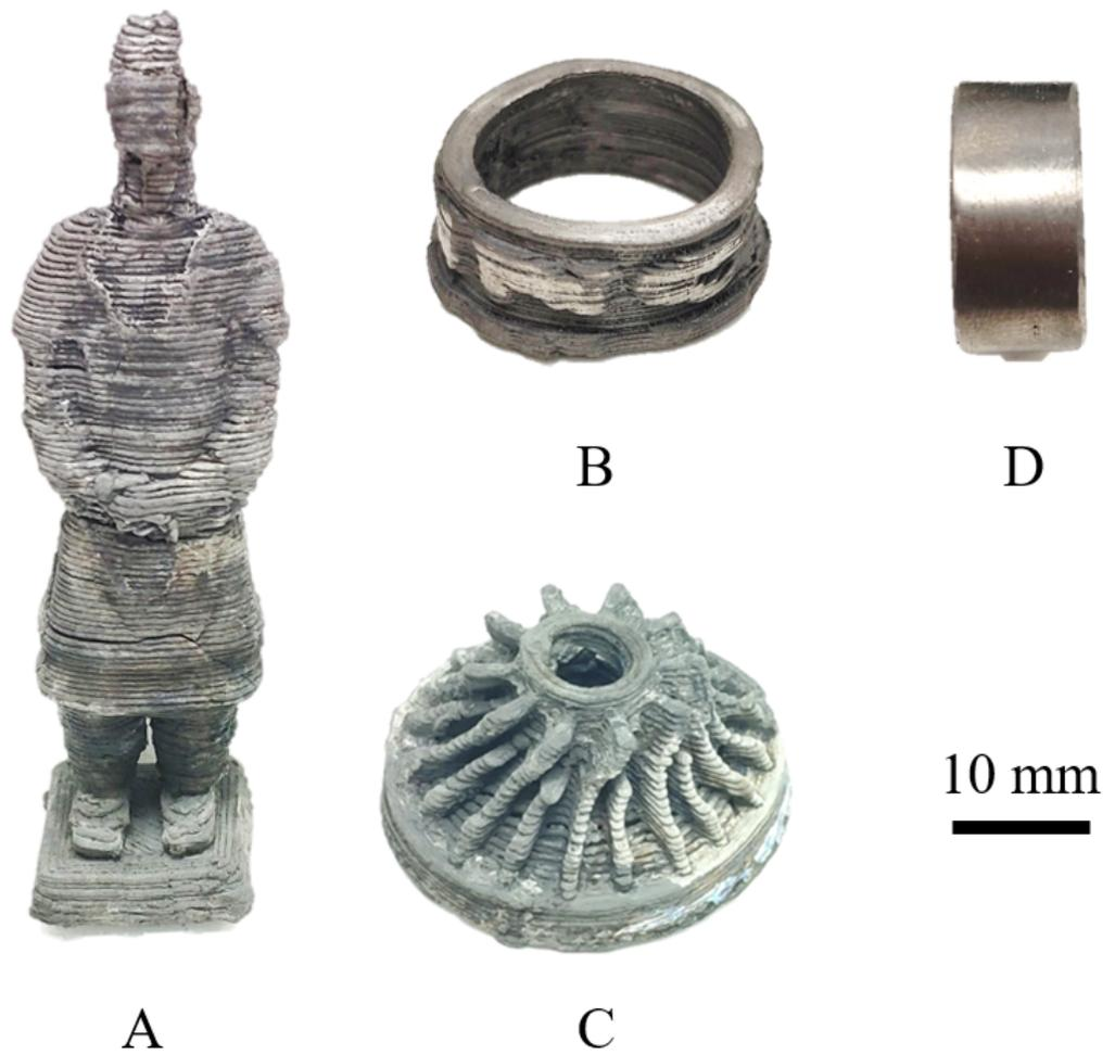
**Figure 5.21:** Examples of the titanium products produced via the NEM Process. A- the Terracotta warrior; B - the “UNNC” labelled ring; C - the impeller with thin vanes/blades; D - the simple polished ring.
