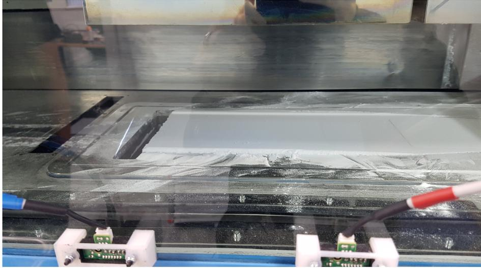
**Figure 5.3.** The optical distance sensors for triggering the measurement process. Sensors were placed in custom 3D printed housings and the housings were attached to the glass access door with double sided adhesive tape.
