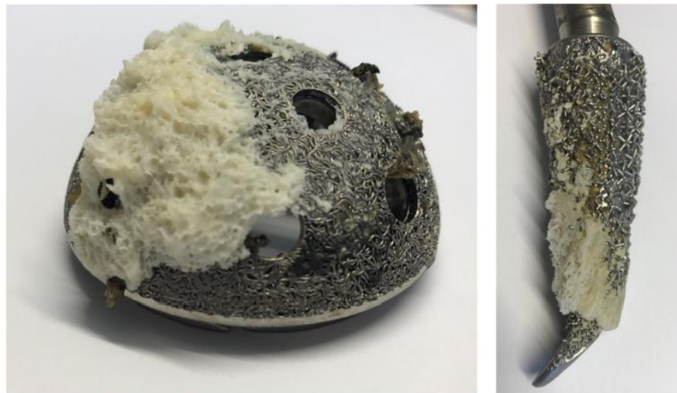
Figure 2:6 Extent of integration due to macro- and micro-structured titanium implants. It is clear that the higher surface area leads to higher implant-to-bone strength, resulting in intra-bone fracture during removal. Images taken from Jäger et al. [97].
