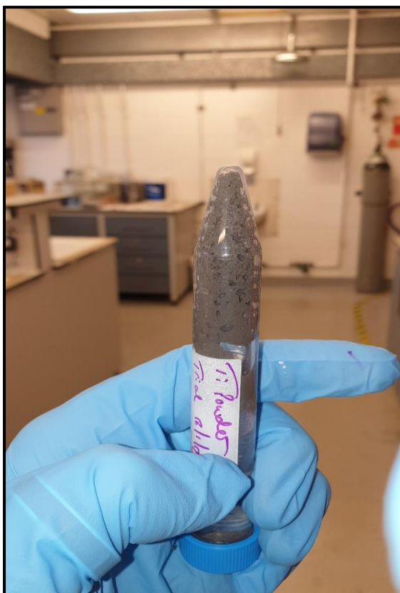
Figure 5:32. Titanate converted Ti microspheres within a polypropylene Falcon tube, exhibiting agglomeration and 'self-assembly' despite agitation of the solution.
